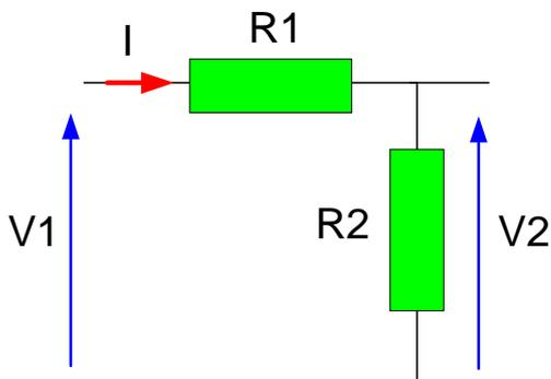
$$V_2 = \frac{R_2}{R_1 + R_2} V_1$$
