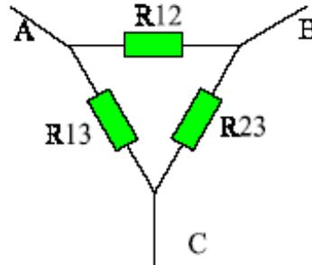
$$R_1 = \frac{R_{12} R_{13}}{R_{12} + R_{13} + R_{23}}$$
