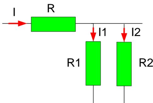
$$I_1 = \frac{R_2}{R_1 + R_2} I$$
